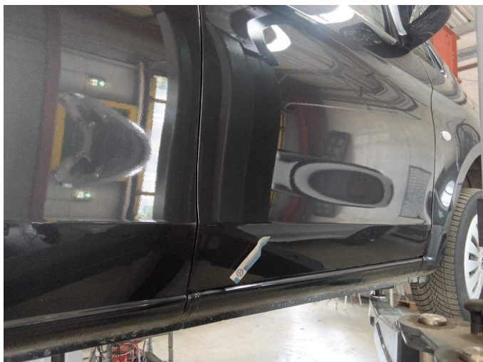
Damage 1: Door - front right side: Door (2) - dent(s) - Lacquer
