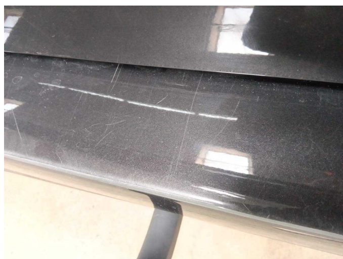
Damage 4: Rear bumper: Rear bumper - Scratch(es) - Paint
