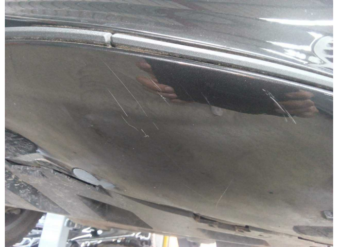
Damage 5: Front bumper: Front bumper - Scratch(es) - Paint
