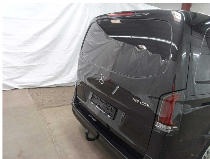
Damage 3: Boot lid / rear door: Boot lid (5) - dent(s) - Smooth repair work
