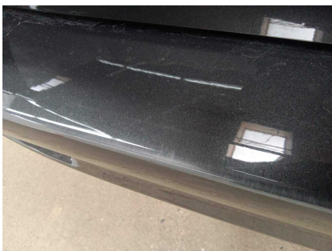
Damage 4: Rear bumper: Rear bumper - Scratch(es) - Paint
