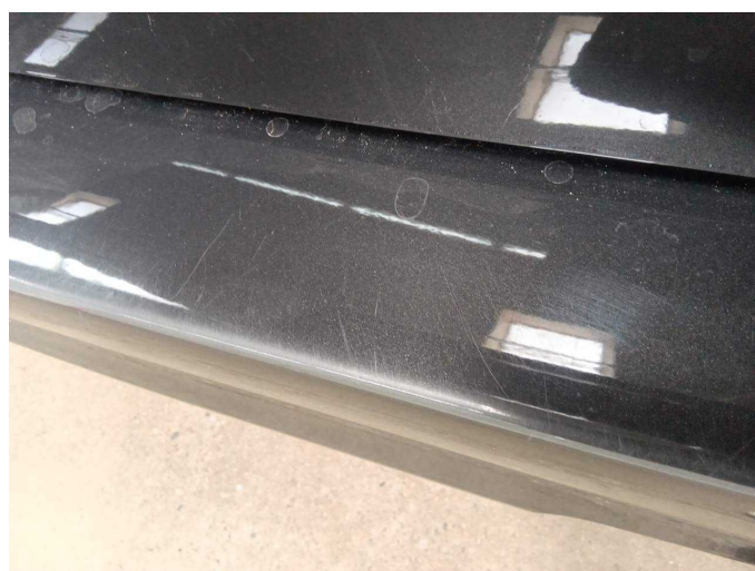
Damage 4: Rear bumper: Rear bumper - Scratch(es) - Paint
