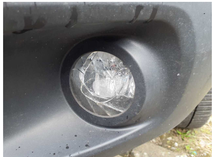
Damage 6: Fog lamp: Fog lamp - front left side - Broken / torn - Replace
