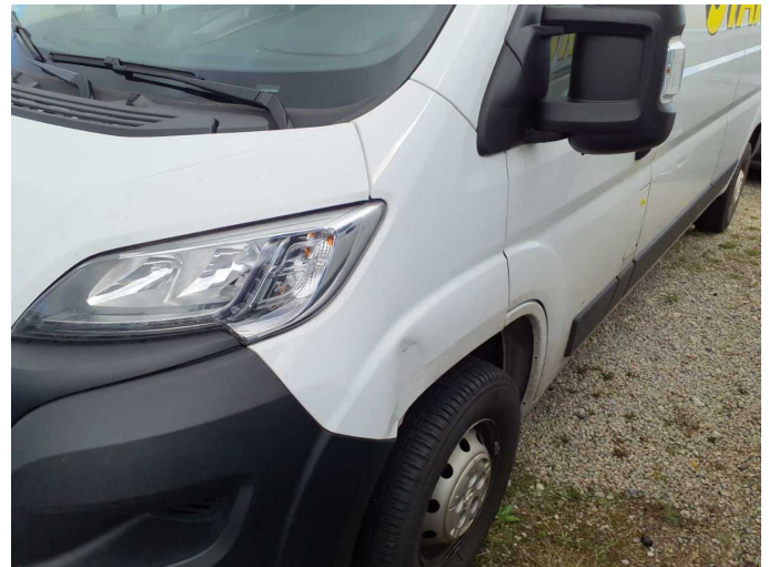
Damage 12: Mudguard - left side: Mudguard - left side - Deformed - Replace
