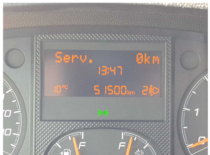
Damage 9: Misc.: Inspection / maintenance - Due - Perform
