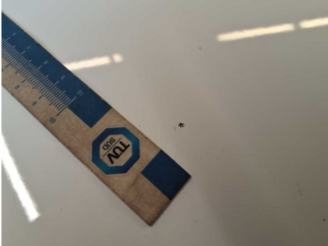
Damage 10: Bonnet: Bonnet - Stone chips - Paint
