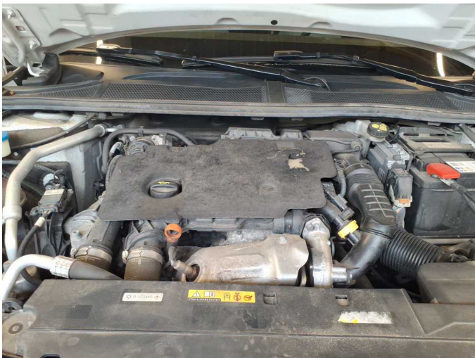
Damage 7: Engine: Engine cover - Damage caused by marten / rodent - Replace
