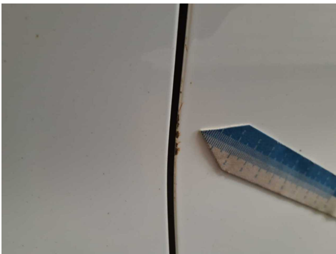
Damage 1: Door - front right side: Door edge - Scratched - Smart repair
