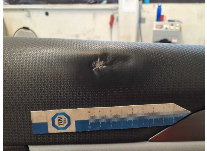
Damage 8: Trim / covers: Door trim - front left side - Broken / torn - Replace
