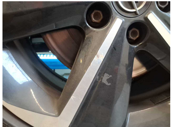
Damage 6: Wheel / tyres: Alloy rim - front right side - Corrosion - Loss in value
