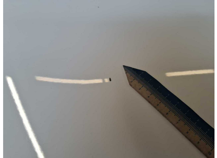
Damage 10: Bonnet: Bonnet - Stone chips - Paint
