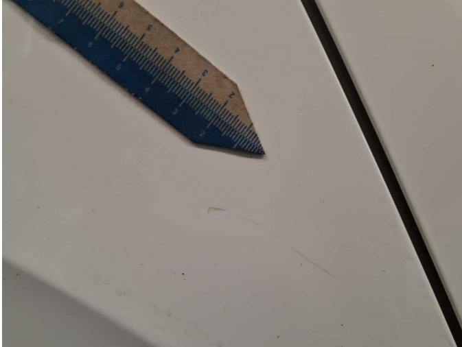
Damage 11: Side panel - rear right side: Side panel - Scratched - Paint
