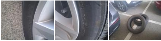
Tyres, Out of tolerance, Replace
