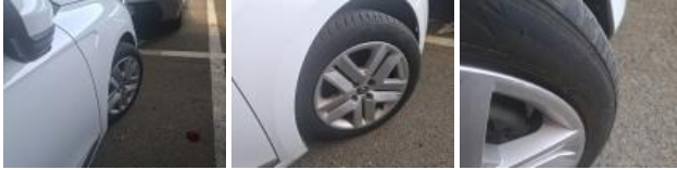
Tyre FL, Out of tolerance, Replace
