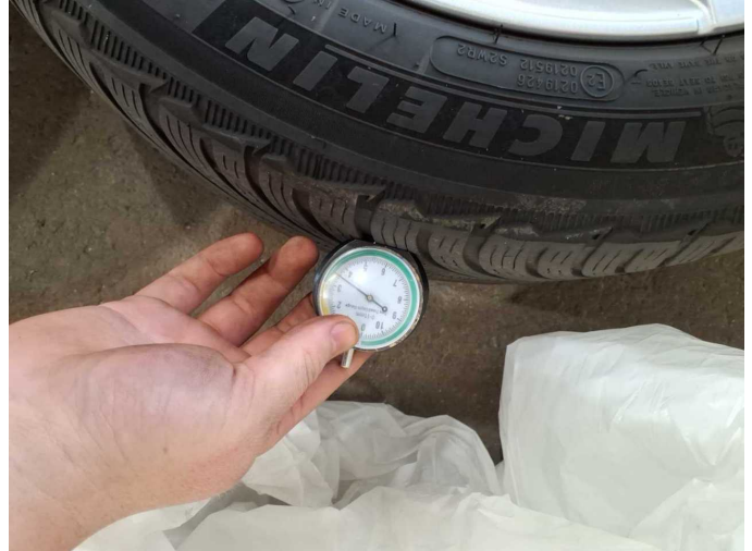
Damage 3: 2nd wheel set: 1 tyre - Worn - Replace
