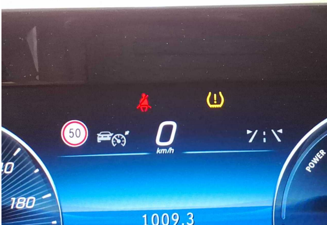
Damage 1: Instrument panel: Indicator light (Reifendruck Kontrollleuchte) - on - Perform diagnosis
