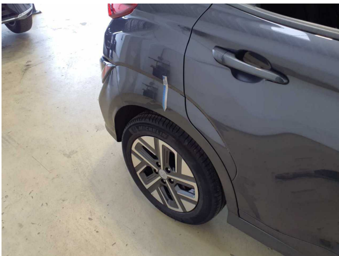
Damage 4: Side panel - rear right side: Wheel well extension (Anätzung) - Paint defect - Smart repair
