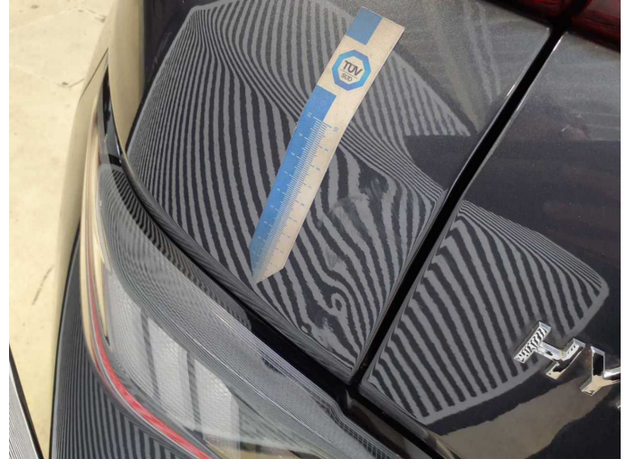
Damage 5: Side panel - rear left side: Side panel - Dent / paintcoat damage - Paint
