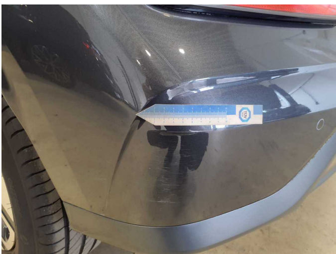
Damage 7: Rear bumper: Rear bumper - Scratch(es) - Paint
