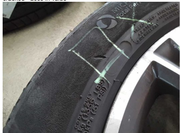
Damage #3: 2nd wheel set: 1 tyre - Damaged - Replace
