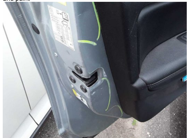
Damage #9: Door - front left side: Door (innen) - Dent / paintcoat damage - Repair and paint
