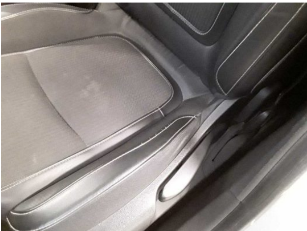
Damage #2: Seat - front: Seat cover - left side - Porous / cracked - Loss in value
