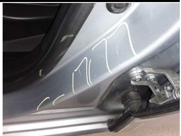
Damage #6: Sill - left side: Sill - Dent / paintcoat damage - Repair and paint
