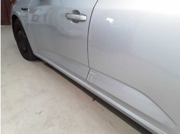
Damage #1: Door - rear left side: Door - Abrasion - Cover / polish
