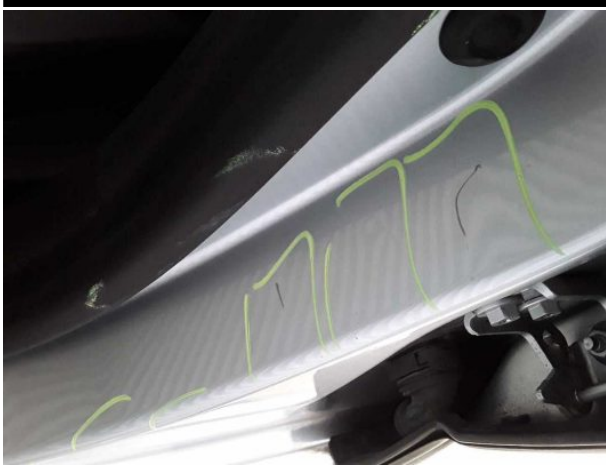
Damage #6: Sill - left side: Sill - Dent / paintcoat damage - Repair and paint
