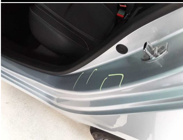
Damage #4: Side panel - rear left side: Sill - Dent / paintcoat damage - Smart repair
