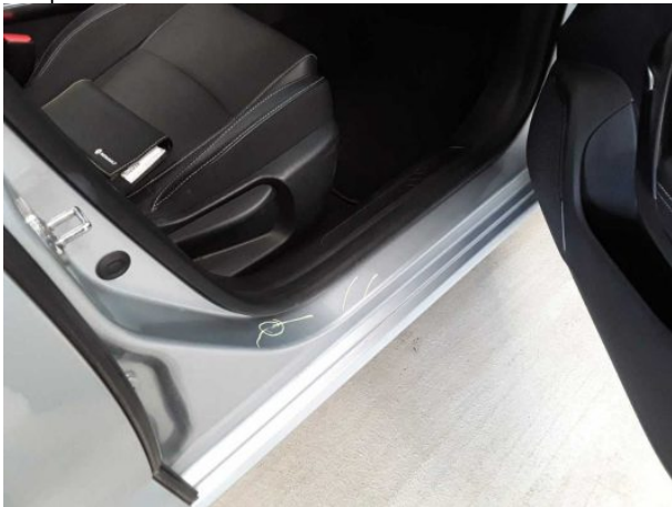
Damage #7: Sill - right side: Sill - Dent / paintcoat damage - Repair and paint
