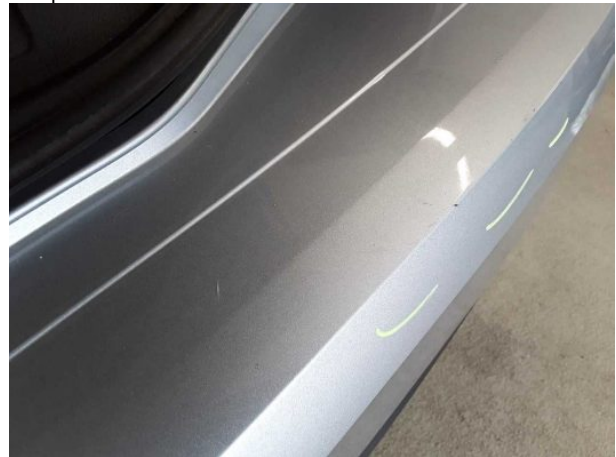
Damage #8: Rear bumper: Rear bumper - Scratched - Repair and paint
