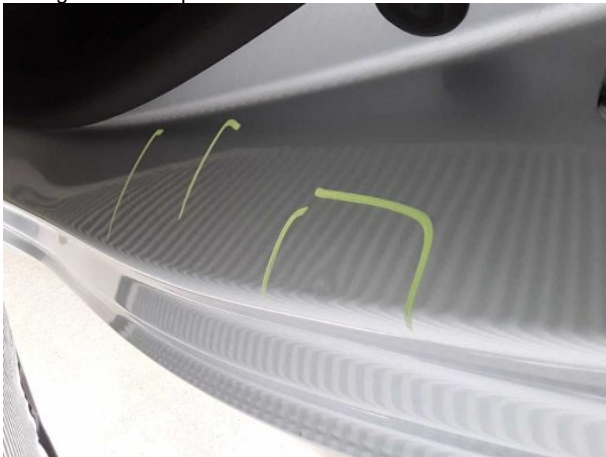
Damage #4: Side panel - rear left side: Sill - Dent / paintcoat damage - Smart repair
