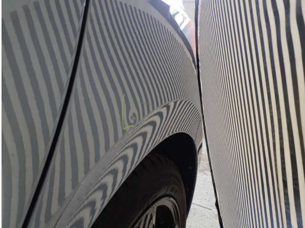
Damage #4: Side panel - rear left side: Side panel - dent(s) - Smooth repair work
