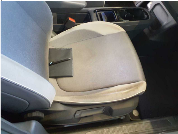
Damage #2: Seat - front: Seat cover - right side - Abrasion - Clean
