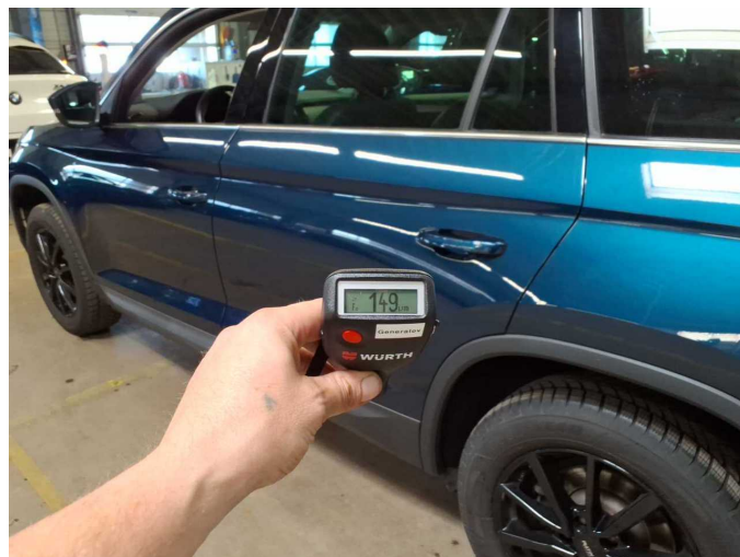
Repainting 3: Door - rear left side
