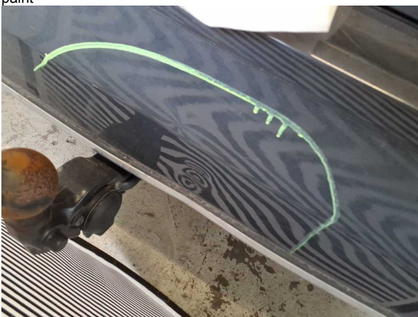
Damage #9: Front bumper: Front bumper - Deformed - Replace
