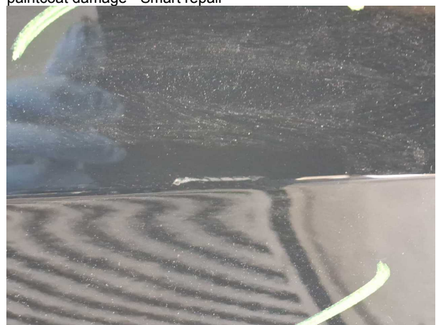
Damage #7: Door - rear left side: Door - Scratch(es) - Repair and paint
