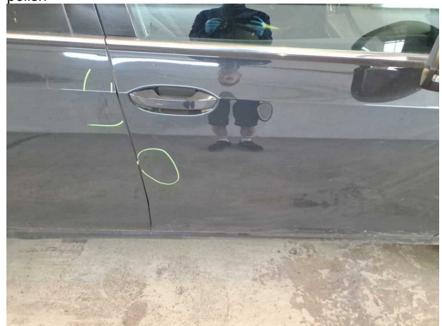
Damage #2: Door - front right side: Door - Dent / paintcoat damage - Smooth repair work
