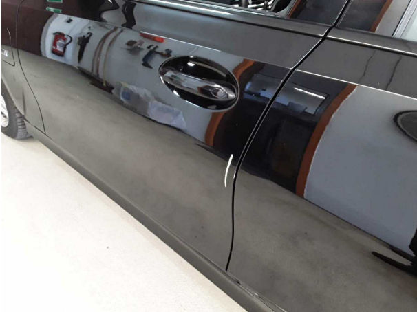
Damage #4: Door - front left side: Door - Scratched - Smart repair
