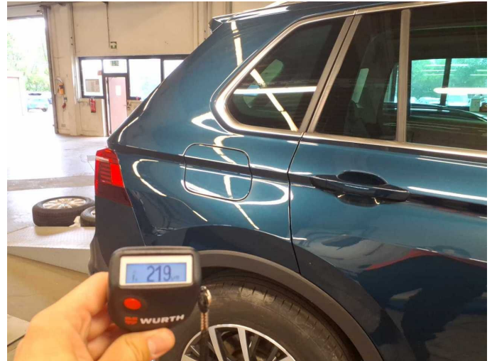
Repainting 5: Side panel - rear right side
