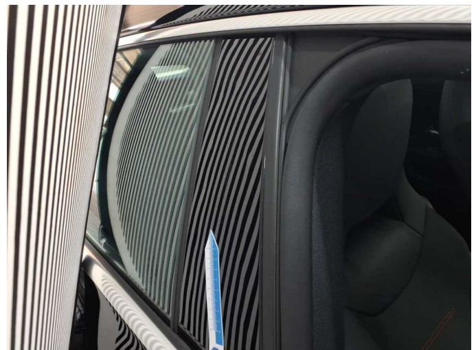
Damage 4: Door - front right side: Window guide (3 dellen) - dent(s) - Replace
