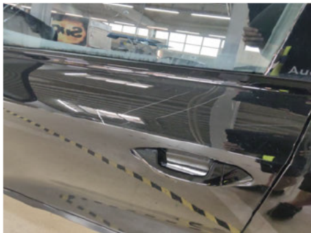
Tür / Vorne Links / Kratzer
