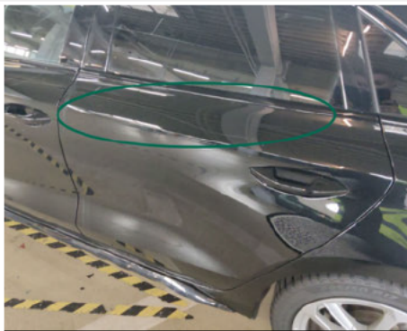
Tür / Hinten Links / Kratzer
