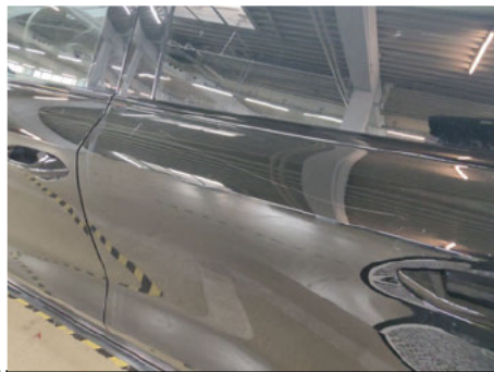
Tür / Hinten Links / Kratzer
