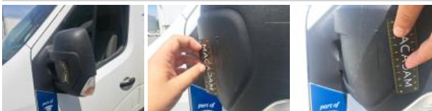
Side panel moulding L, Scratch(es), Replace
