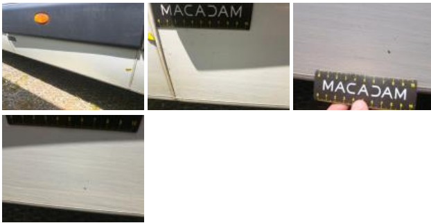
Side panel moulding L, Broken, Replace
