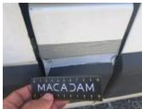
Side panel R, Dent(s) and scratch(es), Repair and paint (complete)
