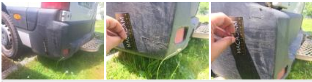
Rear light L, Broken, Replace
