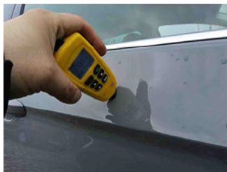
Paint thickness Door FR
