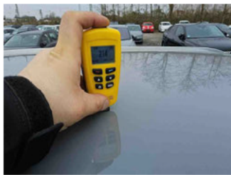
Paint thickness Roof
