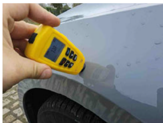
Paint thickness Wing FL
