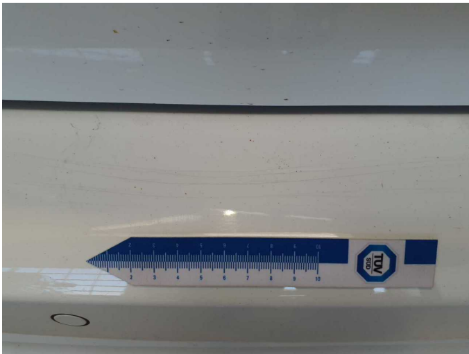
Damage 2: Rear bumper: Rear bumper (Lack gebrochen) - Paint defect - Repair and paint
