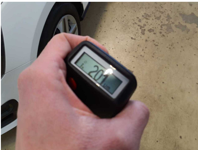
Repainting 1: Mudguard - left side, Door - rear left side, Door - front left side
