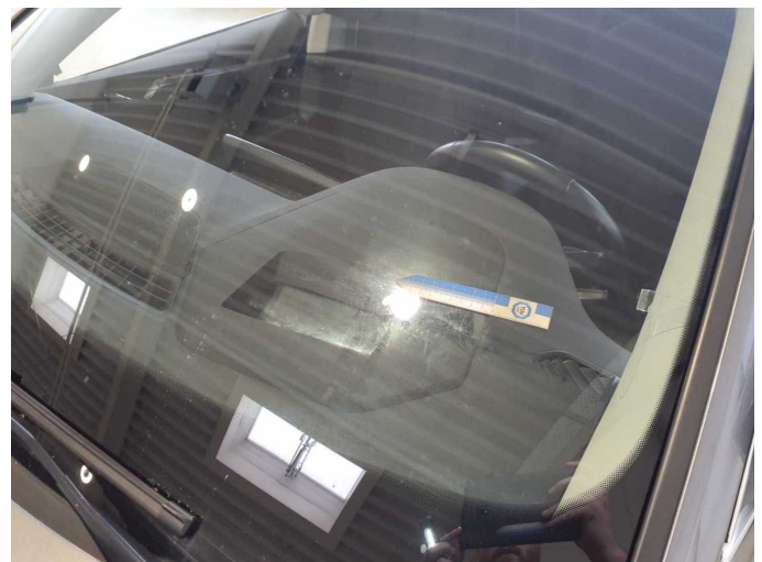
Damage 5: Vehicle glazing: Windscreen - Stone chips - Replace
