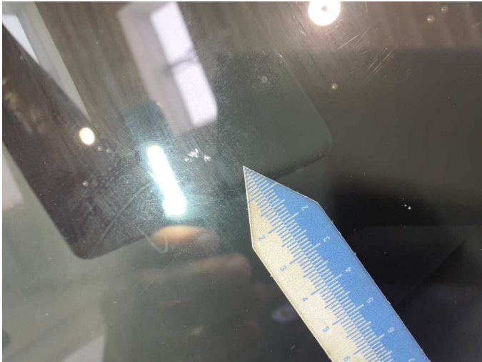
Damage 5: Vehicle glazing: Windscreen - Stone chips - Replace
