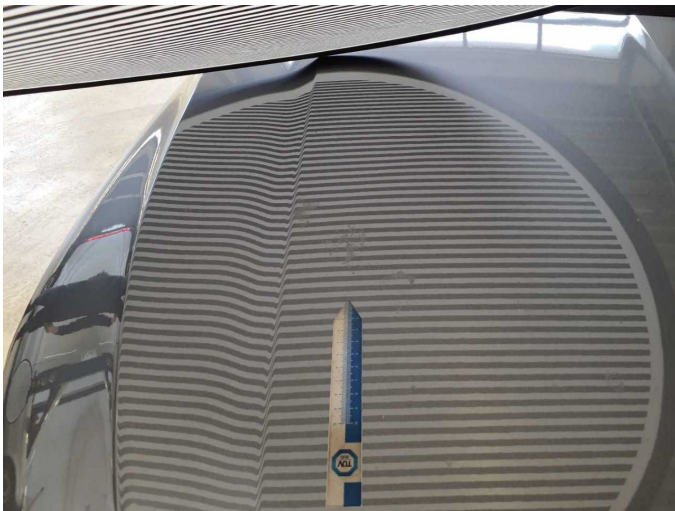
Damage 4: Bonnet: Bonnet - Paint defect - Repair and paint
