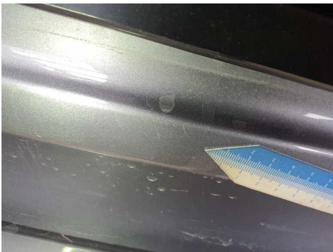
Wear and tear 1: Boot lid / rear door: Boot lid - Scratch(es) - No deduction
