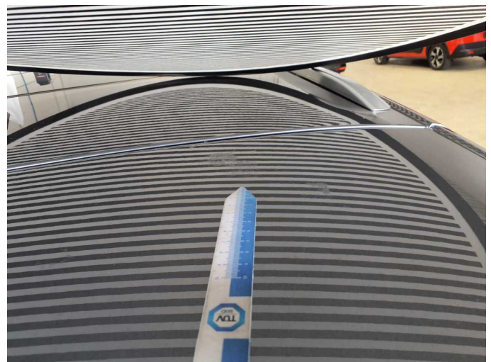
Damage 2: Boot lid / rear door: Rear spoiler (Anätzung) - Paint defect - Repair and paint
