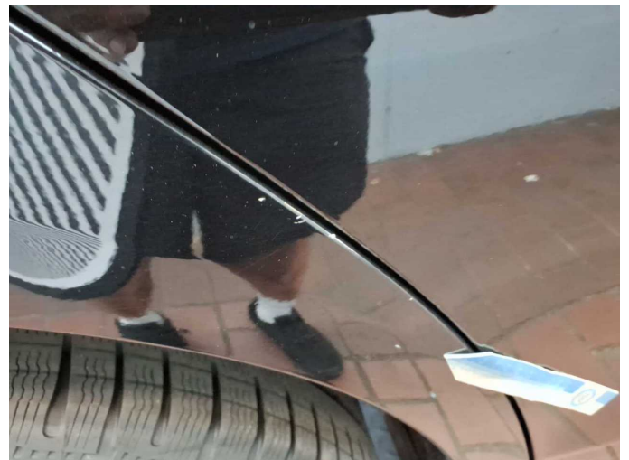
Damage 6: Side panel - rear right side: Elbow - Dent / paintcoat damage - Smart repair
