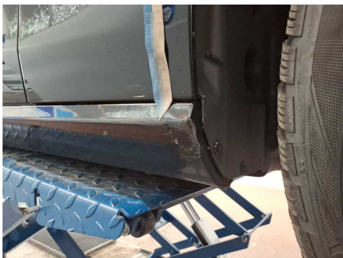
Damage 8: Sill - right side: Trim - Scratched - Replace
