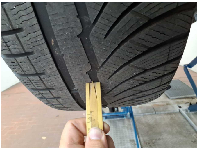
Damage 7: Wheel / tyres: Tyre - right - Does not meet the leasing specifications - Replace
