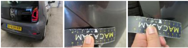
Roof, Dent(s), Repair and paint (complete)
