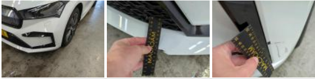
Bumper moulding FL, Broken, Replace and paint
