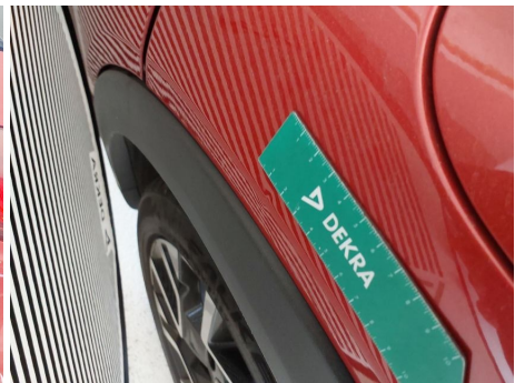
Kotflügel / Hinten Links / Delle
