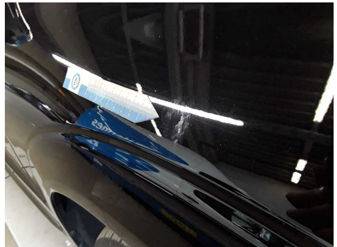
Damage 5: Mudguard - right side: Mudguard - right side (Anätzung) - Paint defect - Paint
