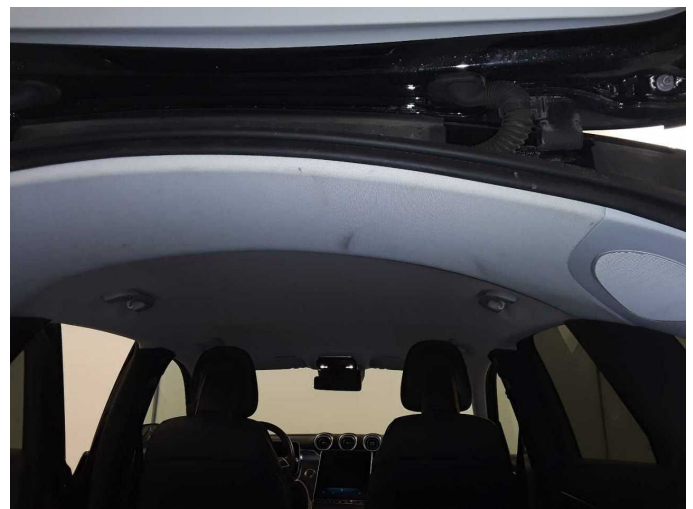
Damage 4: Trim / covers: Roof lining - Soiled - Clean
