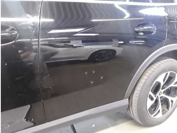
Damage 7: Door - rear left side: Door (4x) - dent(s) - Smooth repair work
