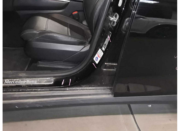
Damage 10: Sill - left side: Sill (+ Aufkleber) - Dent / paintcoat damage - Smart repair
