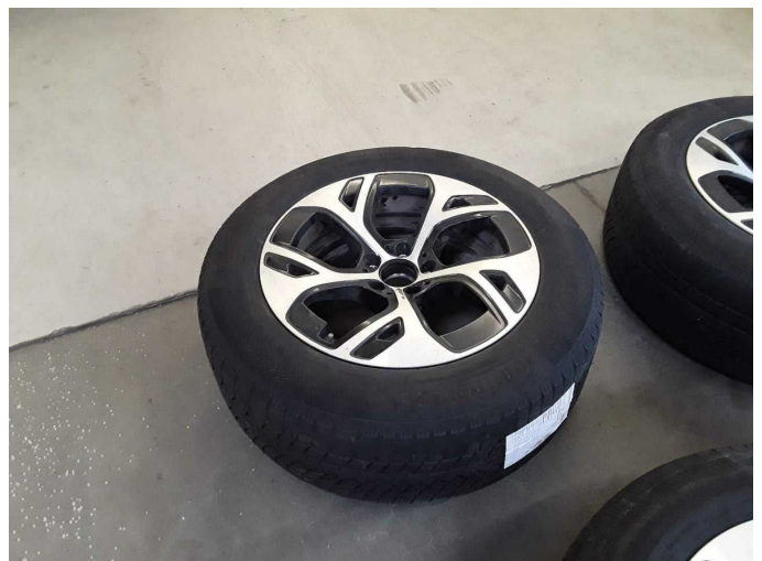
Damage 13: 2nd wheel set: 2 tyres (3mm) - Does not meet the leasing specifications - Replace
