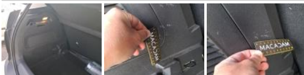
Internal boot lining L, Scratch(es), Replace
