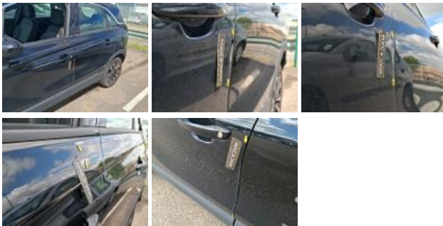
Door RL, Dent(s) and scratch(es), Acceptable
