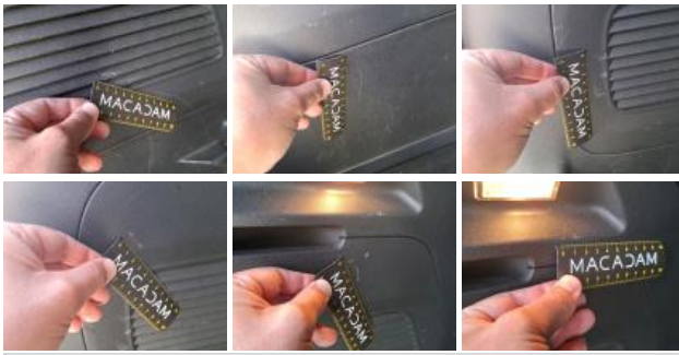
Internal boot lining R, Scratch(es), Replace
