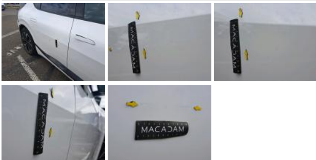
Door FR, Dent(s), Repair and paint (complete)
