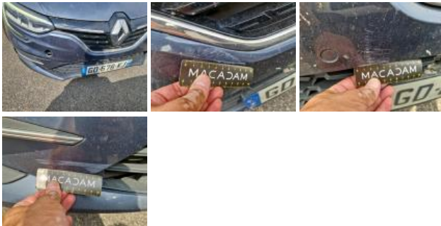
Shutter / cover F, Missing, Replace
