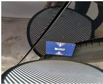
Wing Rear Left // Repair & Painting-scratch + dent
