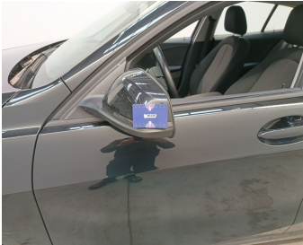
Side View Mirror Left // Replace Not Painted-scratch
