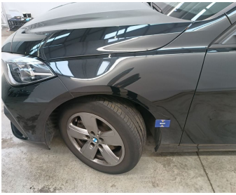
Wing Front Left // Repair & Painting-scratch + dent
