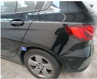
Wing Rear Left // Repair & Painting-scratch + dent
