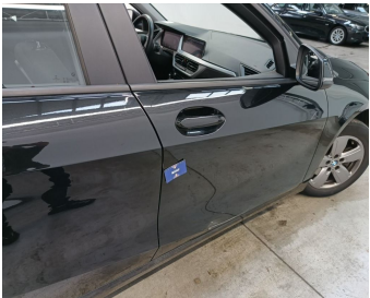
Door Front Right // Repair & Painting-scratch + dent
