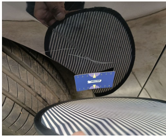
Wing Front Left // Repair & Painting-scratch + dent
