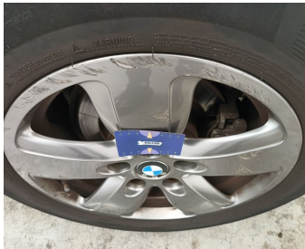
Wheel Alloy Rear Left // Repair-scratch
