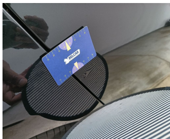
Door Rear Right // Smart Repair Medium-scratch + dent
