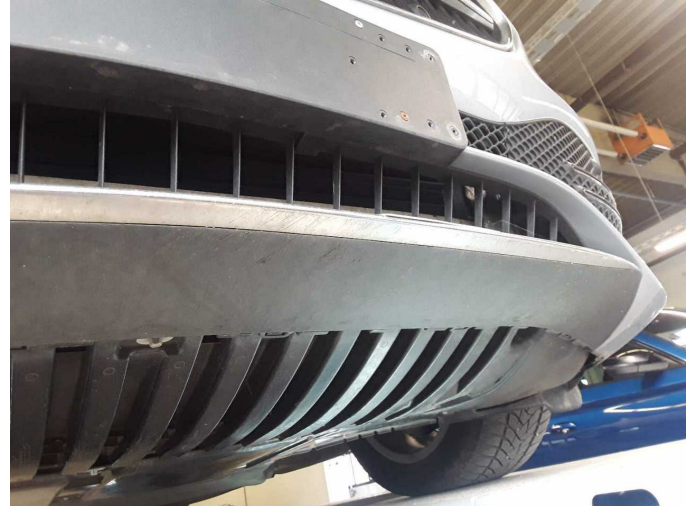
Damage 2: Front bumper: Spoiler (Chromleiste) - Scratched - Replace
