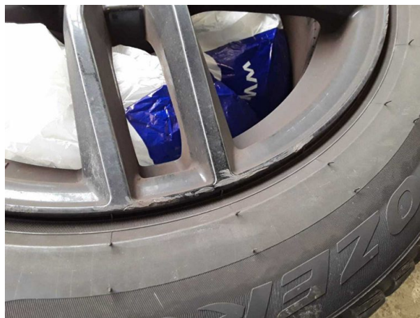
Damage #1: 2nd wheel set: 2 alloy rims - Scratched
