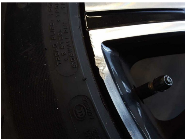
Damage #7: 2nd wheel set: 2 alloy rims - Scratched - Loss in value
