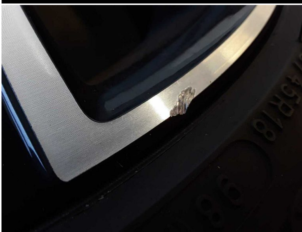
Damage #7: 2nd wheel set: 2 alloy rims - Scratched - Loss in value
