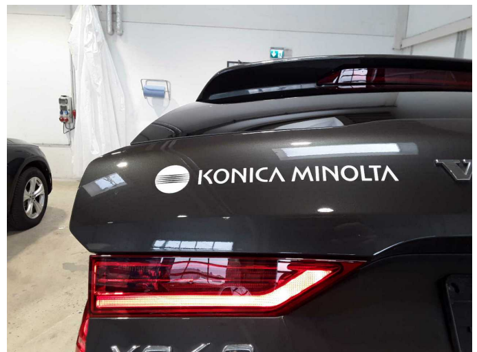
Damage 2: Boot lid / rear door: Boot lid - Glued / labelled - De-glu / neutralise
