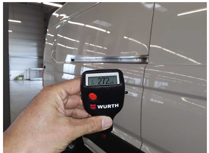
Side panel - rear right side: 272 µm
