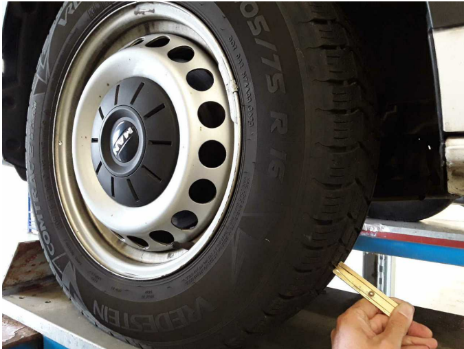
Damage 1: Wheel / tyres: Tyre - front - Does not meet the leasing specifications - Replace
