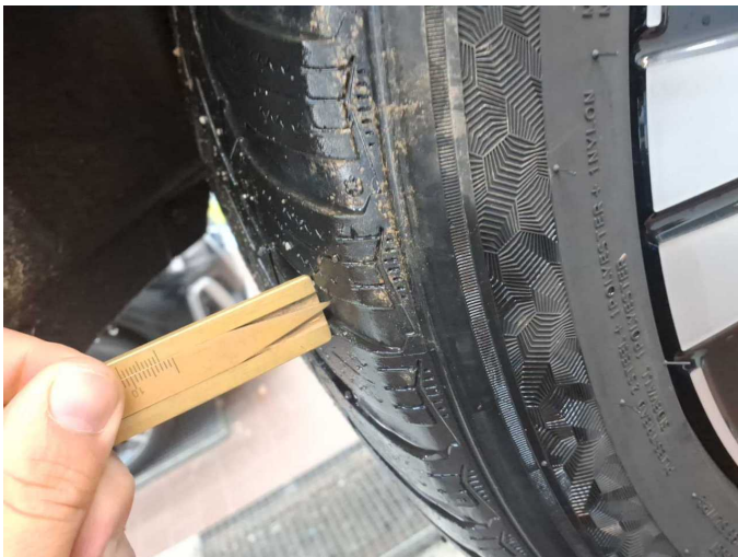
Damage 4: Wheel / tyres: Tyre - right - Does not meet the leasing specifications - Replace
