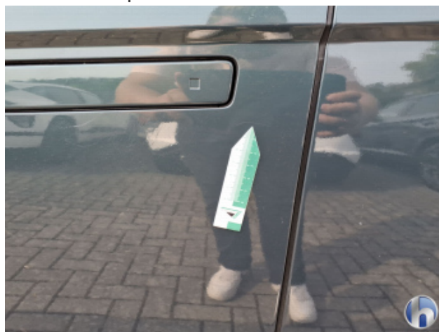
3. Tür Vorne - Links Kratzer - Smart Repair
