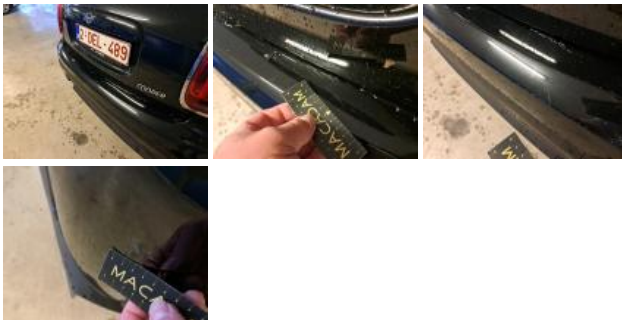
Rear spoiler, Chemical polution, Repair and paint (complete)
