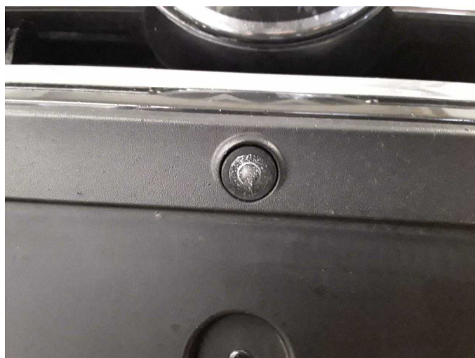
Damage 9: Electronic systems: Front camera - Broken / torn - Replace
