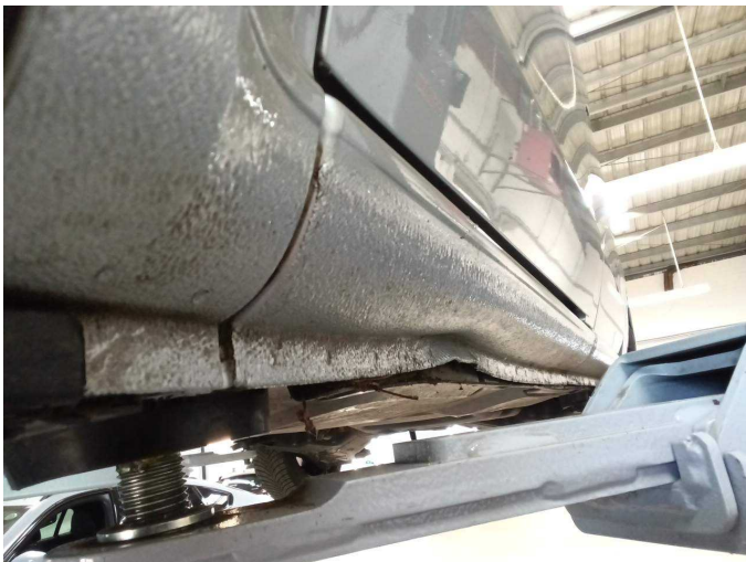
Damage 3: Sill - left side: Sill - Deformed - Repair and paint
