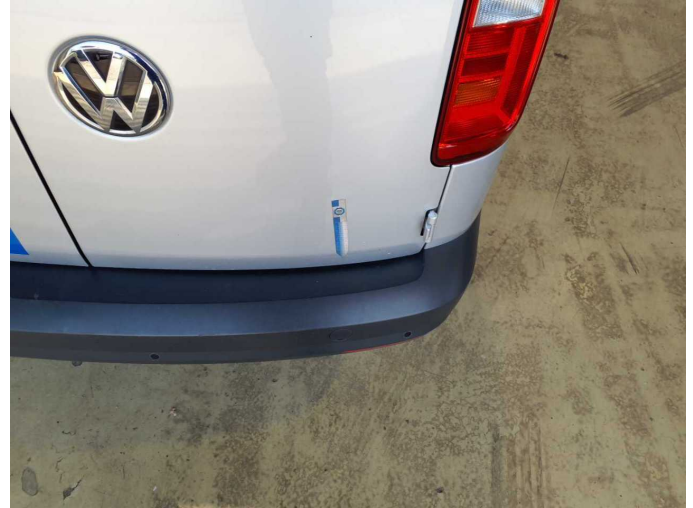
Damage 5: Boot lid / rear door: Rear door - right side - Scratch(es) - Smart repair
