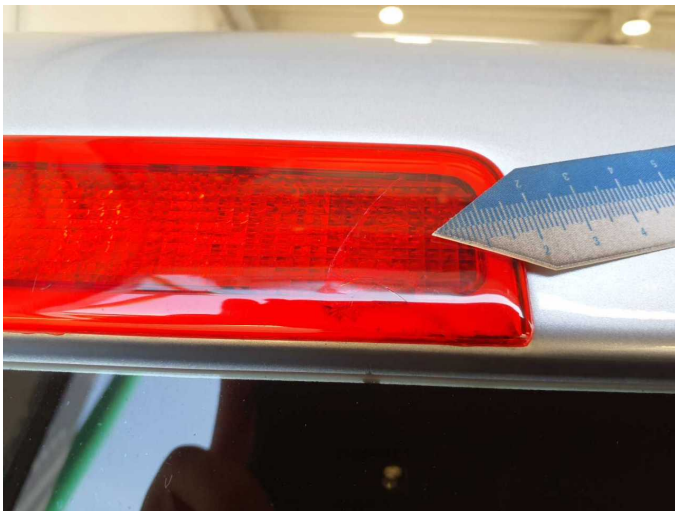
Damage 2: Tail light: Auxiliary brake light - Broken / torn - Replace
