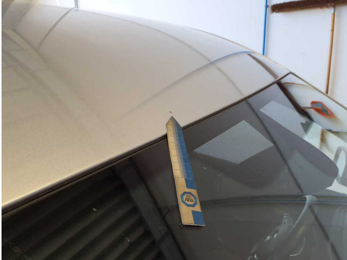
Damage 10: Roof: Roof - Corrosion - Repair and paint
