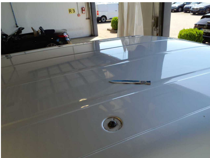
Damage 10: Roof: Roof - Corrosion - Repair and paint
