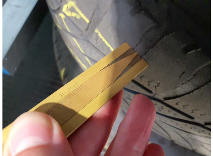
Damage 8: 2nd wheel set: 1 tyre - Worn - Replace
