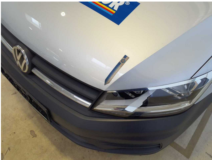
Damage 9: Bonnet: Bonnet - Deformed - Repair and paint
