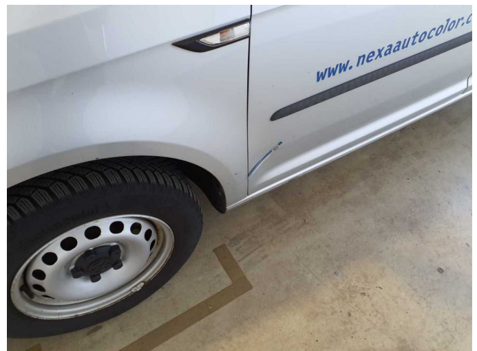
Damage 4: Mudguard - left side: Mudguard - left side - Dent / paintcoat damage - Smart repair
