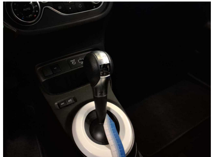
Damage 1: Gearbox: Gear knob - Damaged - Replace
