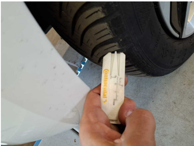
Damage 4: Wheel / tyres: Tyre - front - Does not meet the leasing specifications - Replace
