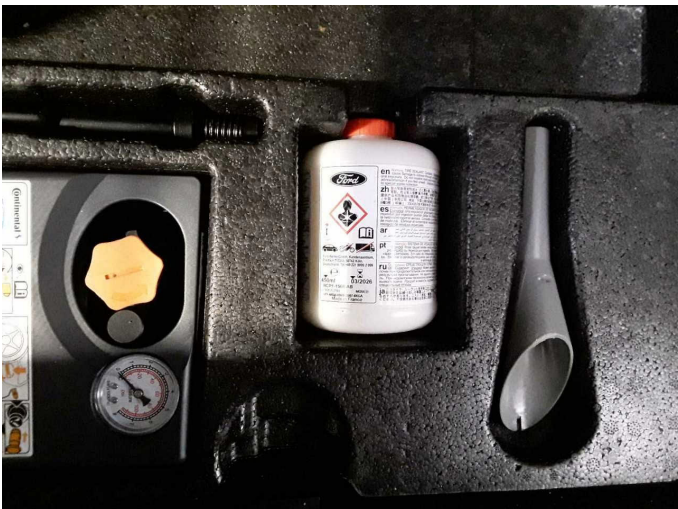
Damage 1: Equipment: Tirefit filler - Expired - Replace
