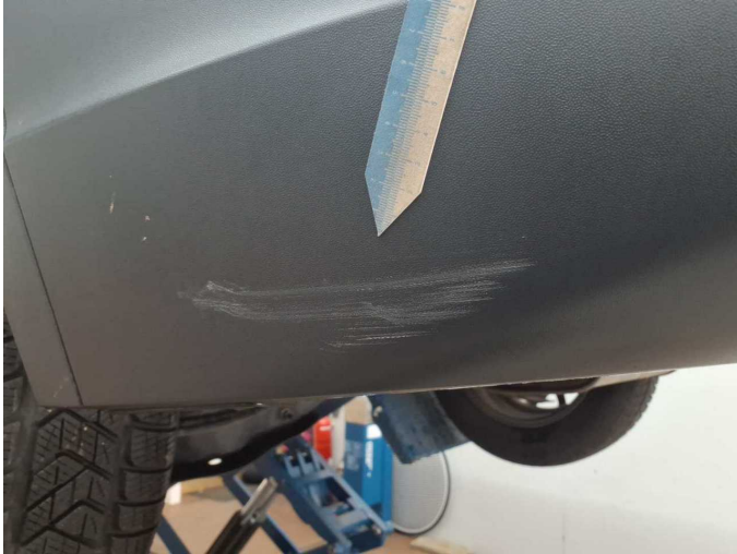
Damage 3: Rear bumper: Spoiler - Scratch(es) - Loss in value
