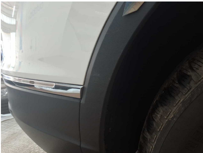
Wear and tear 6: Side panel - rear right side: Wheel well extension - Scratch(es) - No deduction
