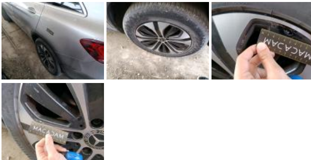
Tyre RR, Out of tolerance, Replace
