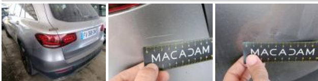
Tailgate / Boot, Dent(s), Repair and paint (complete)
