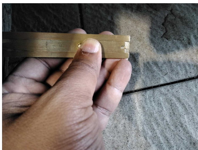
Damage 9: Wheel / tyres: Tyre - front (3mm) - does not meet manufacturer specifications - Replace
