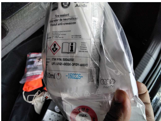
Damage 1: Equipment: Tirefit filler - Expired - Replace
