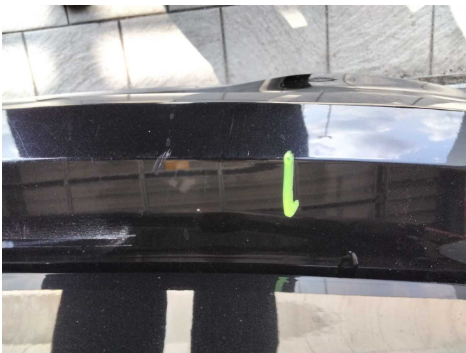
Damage 12: Rear bumper: Rear bumper - Scratch(es) - Paint
