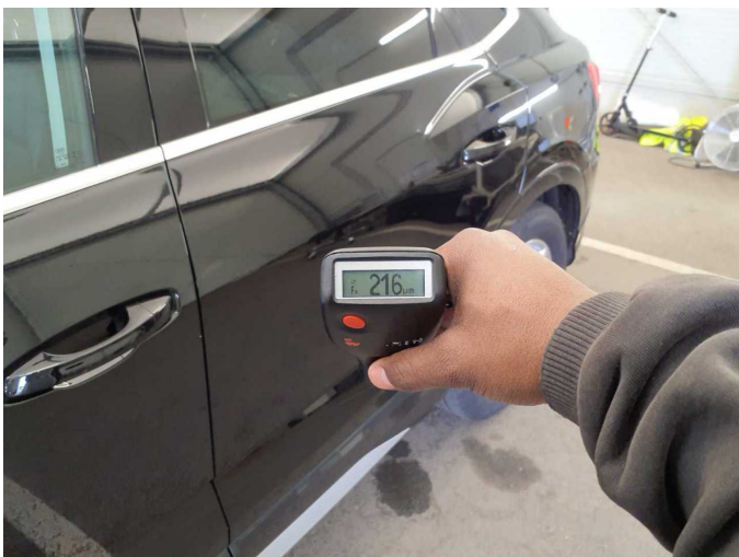
Repainting 3: Door - rear left side
