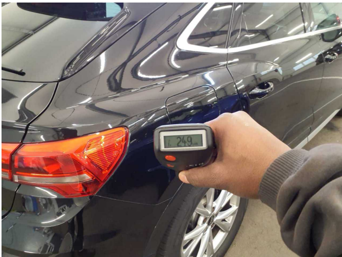
Repainting 2: Side panel - rear right side
