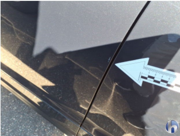
7. Schweller - Links Kratzer - Smart Repair
