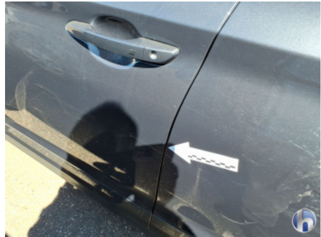
7. Schweller - Links Kratzer - Smart Repair
