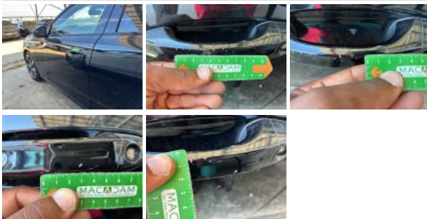
Number plate F, Deformed / Strained, Repair/replace (lump sum)
