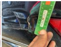
Bumper R, Broken, Replace and paint
