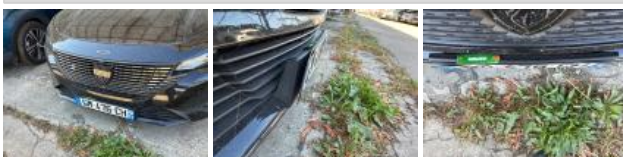
Number plate F, Deformed / Strained, Repair/replace (lump sum)
