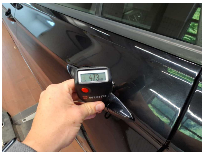
Repainting 3: Door - rear left side
