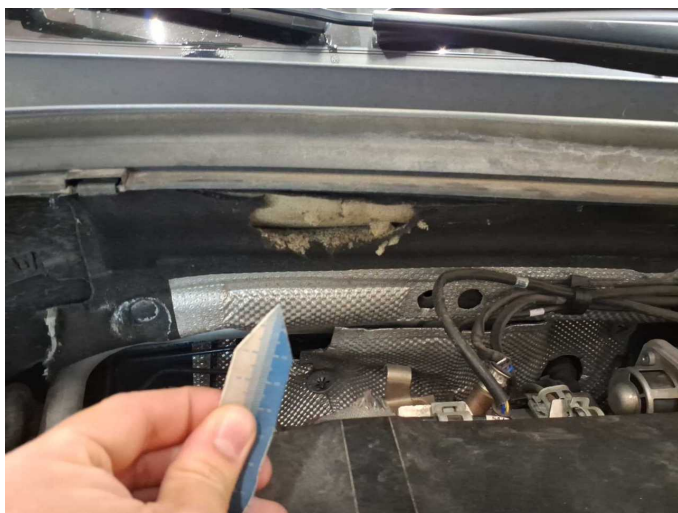
Damage 1: Body: Firewall trim (Dämmmaterial) - Damage caused by marten / rodent - Replace
