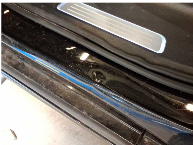
Damage 1: Side panel - rear left side: Sill - dent(s) - Smooth repair work
