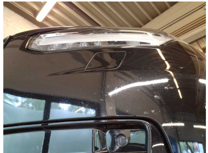
Damage 3: Front bumper: Front bumper (Sandstrahleffekt) - Stone chips - Paint
