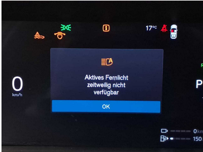
Damage 2: Instrument panel: Indicator light (Abstandhalter+Scheinwerfer) - on - Perform diagnosis
