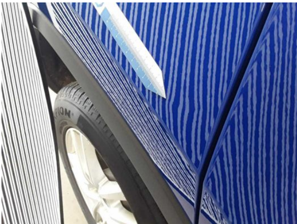
Damage #10: Side panel - rear right side: Side panel (Kratzer) - Dent / paintcoat damage - Repair and paint
