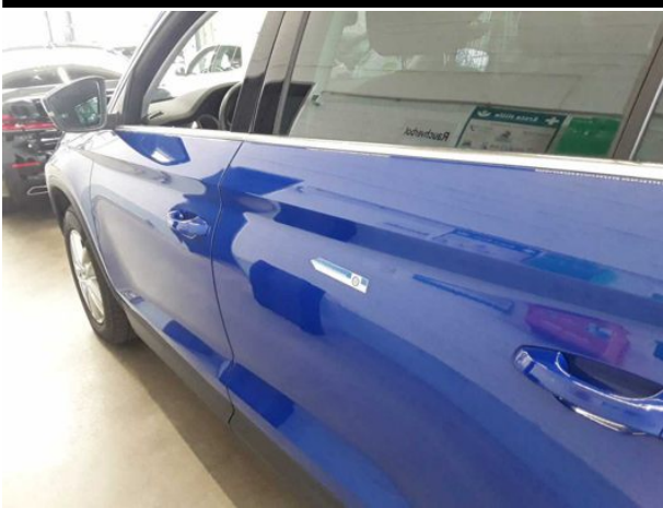
Damage #8: Door - rear left side: Door - Dent / paintcoat damage - Repair and paint
